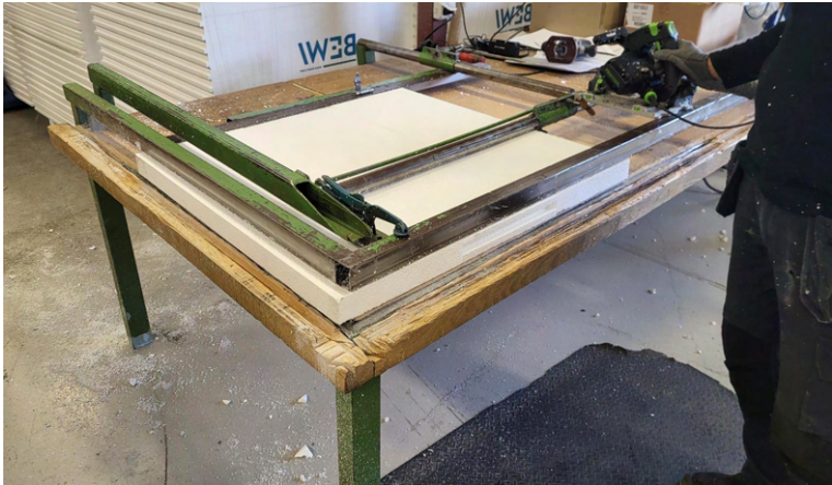
Figure 3.1: The current cutting setup, difficult in operation and causes Styrofoam to be spread in the work area
