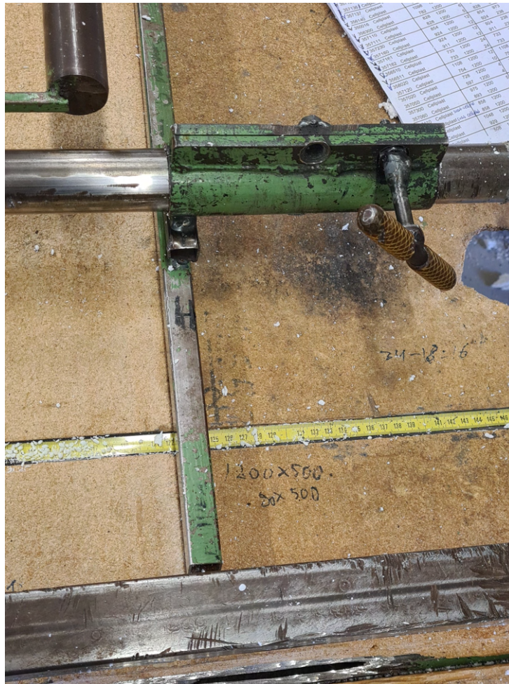
Figure 3.3: Adjustable stop on existing machine set by using the measuring tape to set the cutting position
