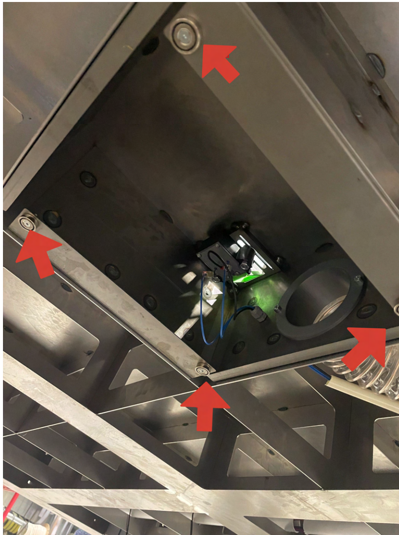
Figure 5.19: The box below the table. The red arrows point to the magnets
