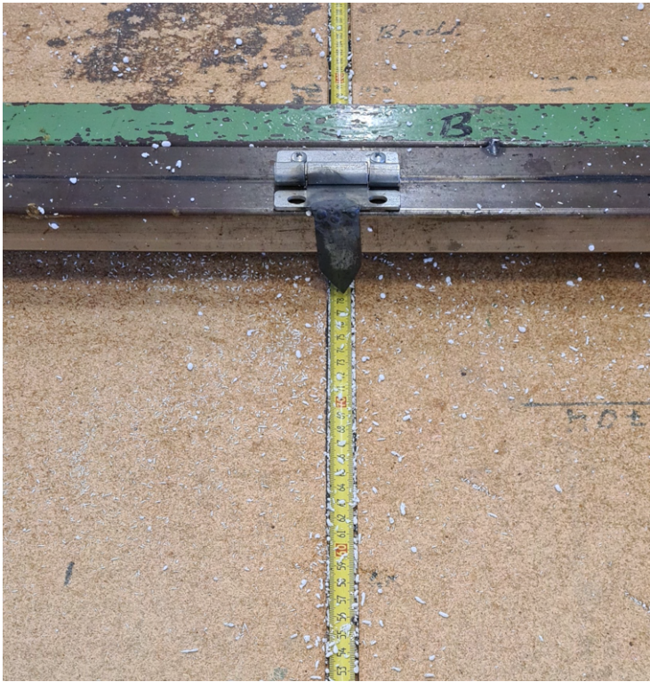
Figure 3.2: Adjustable stop on existing machine where a measuring tape is used to set the cutting position along with an indicator on the machine
