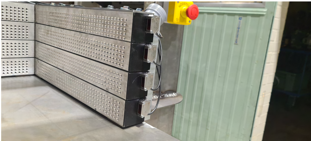
Figure 5.24: Proximity sensors mounted on the end of the Styrofoam holder
