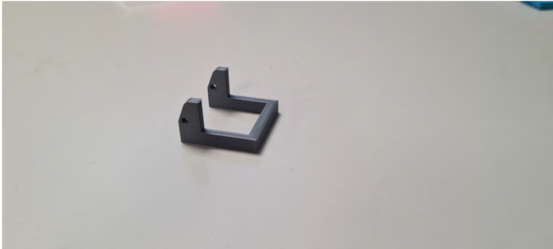
Figure 4.7: A late prototype of the lever used in the clamp for the bottom wire
